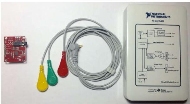
Figure 3. AD8232 ECG module and NI myDAQ card
