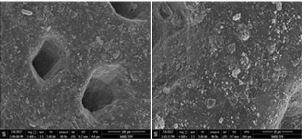
Figure 5. SEM Imagines of 24% TBP Treated Leathers
