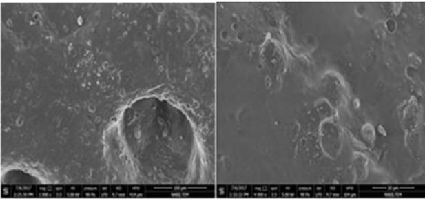
Figure 3. SEM Imagines of 8% TBP Treated Leathers
