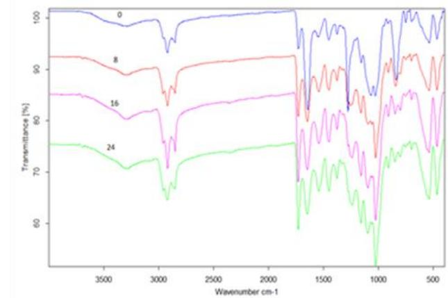
Figure 6. ATR-FTIR Results of TBP Treated Leathers
