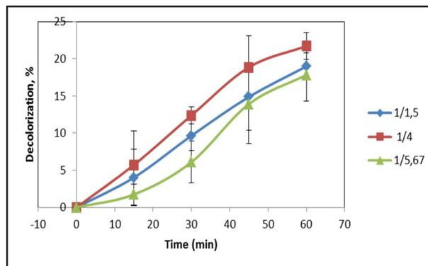
Fig.4. Effect of wastewater dilution ratio on decolorization of baker's yeast effluent (volume=500mL, power=80W, pulsed cycle=30%)
