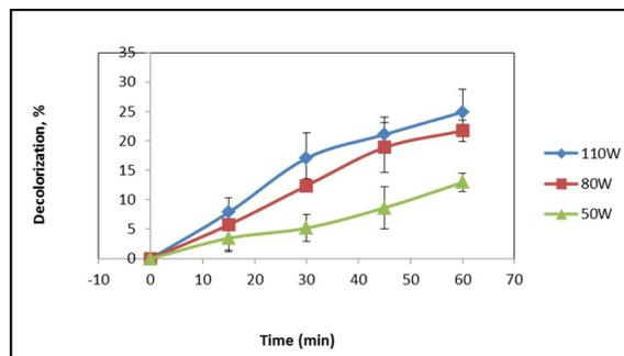
Fig. 2. Effect of ultrasonic power on decolorization of baker's yeast effluent (volume=500mL, dilution ratio=1/4, pulsed cycle=30%)
