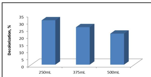
Fig.3. Effect of wastewater volume on decolorization of baker's yeast effluent at the end of 60min reaction time (dilution ratio=1/4, power=80W, pulsed cycle=30%)
