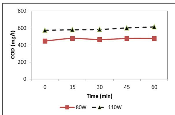
Fig.6. Effect of ultrasonic power on COD removal of baker's yeast effluent (volume= 500mL, dilution ratio=1/4, pulsed cycle=30%)
