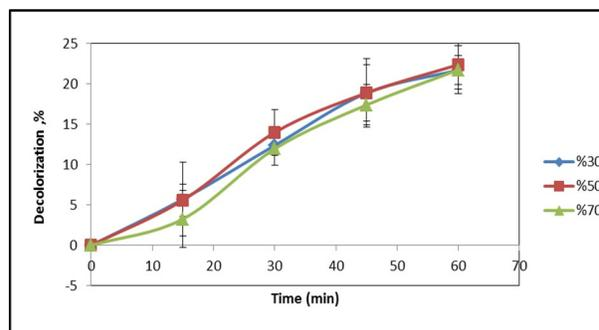
Fig.5. Effect of pulsed cycle on decolorization of baker's yeast effluent (volume= 500mL, power=80W, dilution ratio=1/4)
